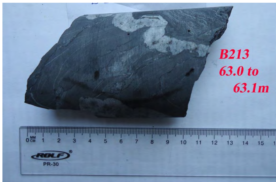
Figure 4-33: Bulk density 2.57 (true density 2.57) V_2O_5\% 0.2 and no carbon analysis (in FW waste zone) DSG19
