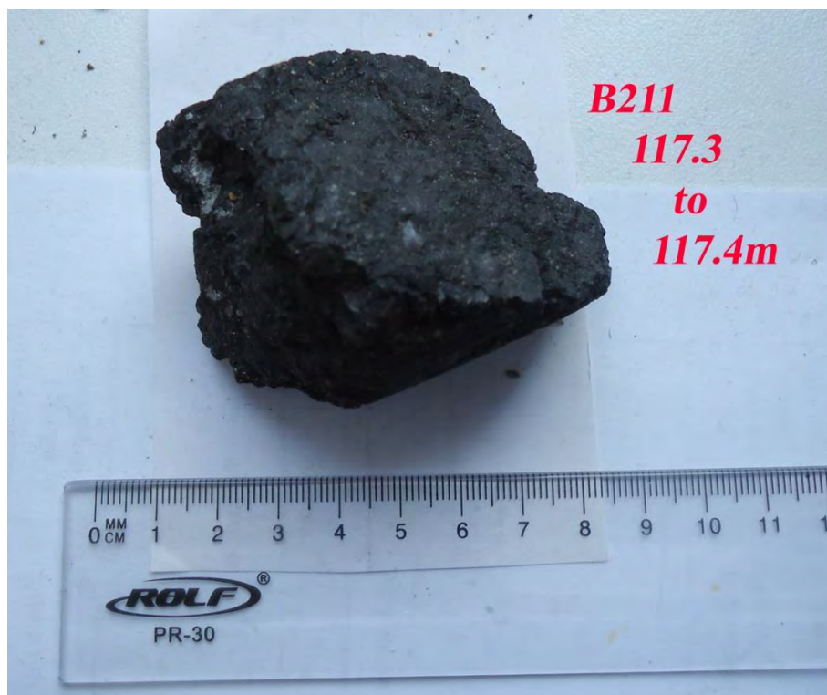
Figure 4-31: Bulk density 2.13 (true density 2.25) V_2O_5 % 0.5 and carbon 22.7 % DSG9
