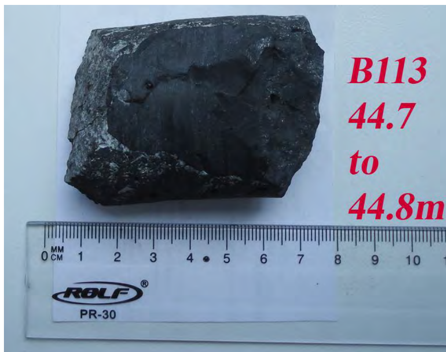
Figure 4-32: Bulk density 2.46, V_2O_5\% 0.75 and carbon 23.0 % (no true density) DSG15
